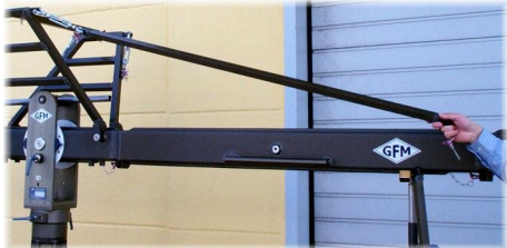
Connecting 2 x 142cm rigging rods to the turnbuckles
