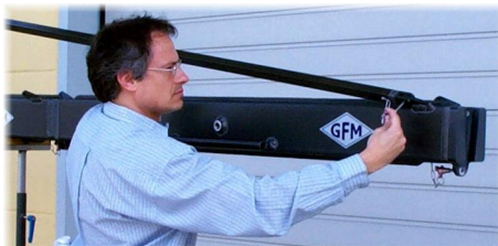
Connect the rigging rod to the end section and secure with a locking pin.
